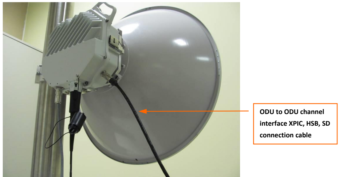
Figure 4.1-10 : Detail of ODU/ODU cable
